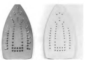
Surface profiling of Iron with silicon carbide improves adhesion of Teflon coating.
