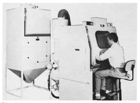
This production blast system includes reclaimer/dust-collection to recycle media and remove dust, debris and fines. Raised work station and padded armrests reduce operator fatigue. (Illustrations courtesy of Empire Abrasive Equipment Co.)
