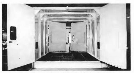
Blast room for processing large parts isolates the blasting from the outside environment. Automatic media-collection/recycling equipment can be included.
