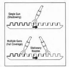
The single gun in the top drawing fails to clean "shadowing" surfaces. Multiple guns (bottom) remedy the problem.
