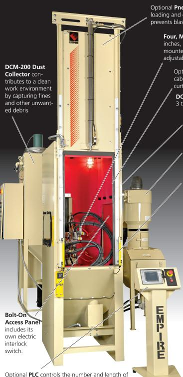
guns oscillations. (Standard control panel mounts on the left side of the cabinet in place of the viewing window.)
