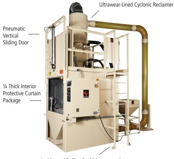
Ladder and Railing for Maintenance Access
