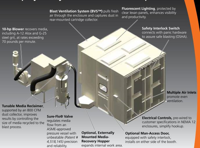
Empire's Pre-Engineered Blast Booths (PEB) feature the essentials of blast rooms at a fraction of the cost. These ten-and-twelve-foot-high booths not only include the hardware required to strip large parts fast. They also reclaim media, remove dust and breathe fresh air into the work enclosure with Empire's exclusive Booth Ventilation System (BVS).
