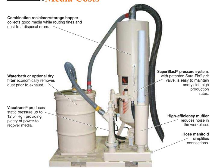
As environmental codes become more stringent, the demand for contained blasting rises. By enabling you to recover media at the nozzle, Empire's Blast N' Vac product line virtually eliminates the need to collect media manually, resulting in safer, cleaner blasting.
