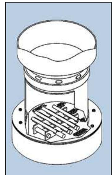
*Similar in design to Empire's PRS, FaStrip portables include special features for assuring smooth flow of plastics and other light media. **Magnetic separator** (shown left) extracts ferrous debris capable of damaging delicate substrates.*
