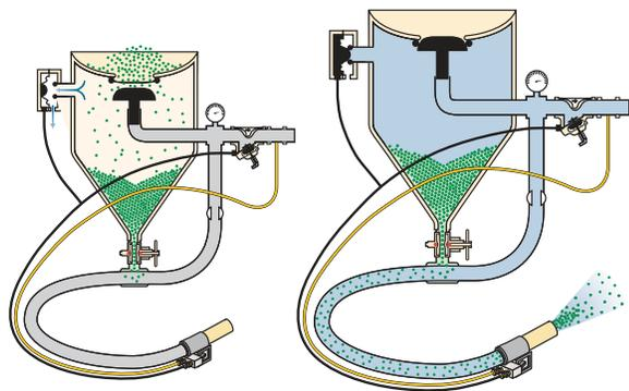
**680 (blow-down) controls**, used on SuperBlast and Econo-Blast portables, vent pressure from the vessel when the “on/off” trigger is released. This setup makes blasting easier for a single operator and permits automatic grit refills.
