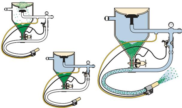
**780 (pot-under-pressure) controls**, used with Empire’s SuperBlast, PRS and FaStrip systems, stop blasting when the “on/off” trigger is released while maintaining pressure in the vessel. This arrangement, which conserves compressed air and is easiest on system components, is especially useful for spot blasting because of the fast restarts it provides.
