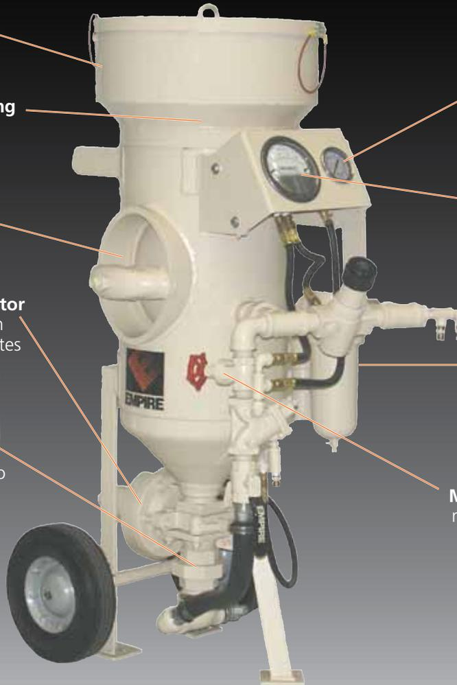
**Blast-pressure gauge** shows operating psi.
