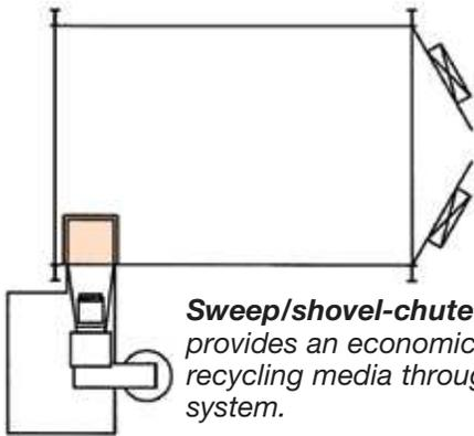
**Sweep/shovel-chute** recovery system provides an economical method for recycling media through the air-wash system.
