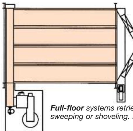
**Full-floor** systems retrieve media more quickly and reduce labor costs by eliminating the need for sweeping or shoveling. Floors exceeding 30' feature a cross module between long modules.
