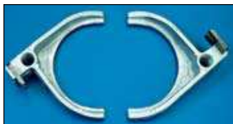
Shifter forks etched with ALOX
