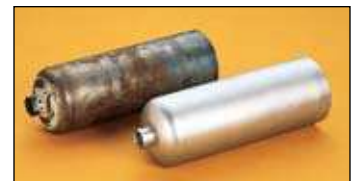
Cylinder surface profiled with ALOX
