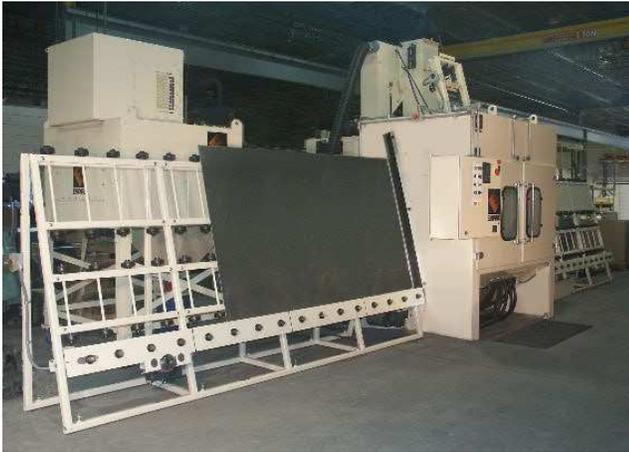
main objective was to produce a uniform blasted surface, on one side, within a self-contained environment.
