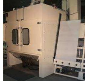
With PLC Automatic System Controls, the unit reduces operator involvement and uniformly blasts each part while keeping him out of harms way. For added control, the process can be stopped and restarted without lose of a uniform finish and finish is maintained across the entire part surface.
