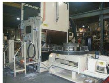
The machine includes part recipe capability, where each part is programmed once and then available for recall. The program provided a 4-step sequence, including an air-only blow-off cycle to complete the process.
