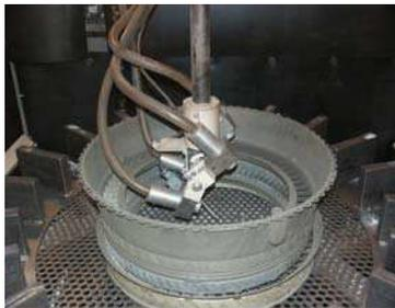
dual-turnstile, 4-axis pressure blast system with state-of-the-art PLC controls. System was further enhanced with a touch-screen display
