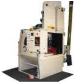
this additional motion, the rotating guns were able to evenly cover the inside and outside table diameters.
