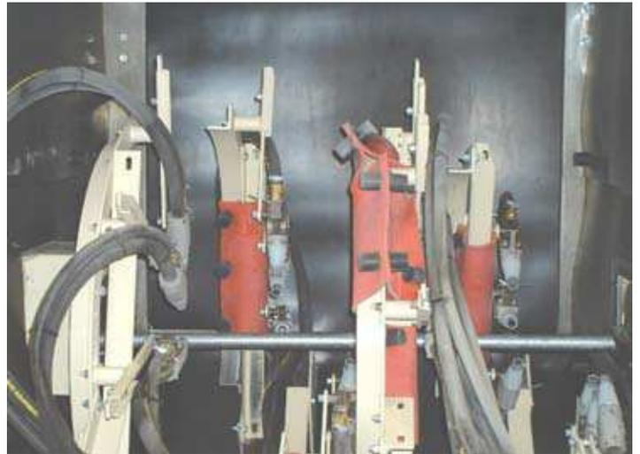
*Empire's automated blast systems remove gloss from and create anchoring profiles on aluminum electrical cables ranging in diameter from one-quarter to three inches. The blast system shown above deploys 12 guns firing plastic pellets to remove gloss from aluminum wire at rates of up to 20 linear feet per minute.*
