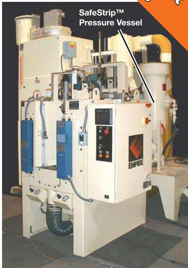
our run-off tests demonstrated variances of less than 0.1% — well within the customer’s tolerance of 5% — while blasting with under four ounces of media per minute.
