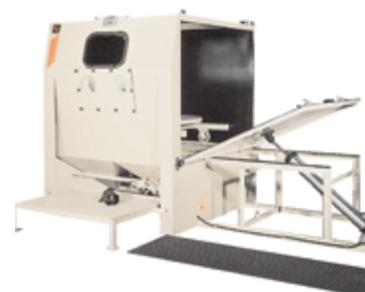
**Heavy-duty Empire cabinet with a work enclosure exceeding 4 cubic meters provides an environmentally friendly and economically attractive approach for air-blasting parts with maximum dimensions of up to 1.8 meters.**
