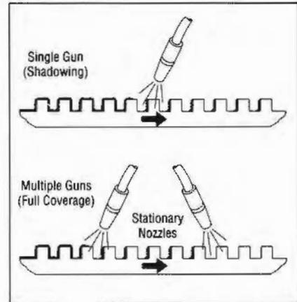
**The single gun in the top drawing fails to clean "shadowing" surfaces. Multiple guns (bottom) remedy the problem.**
