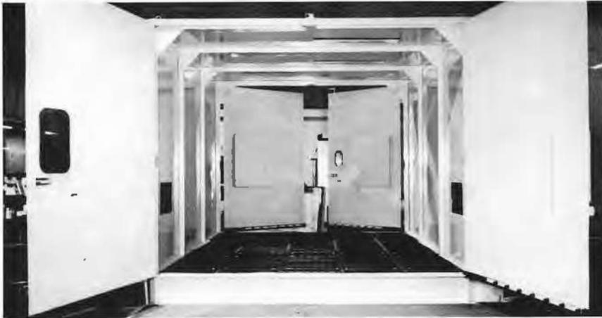
**Blast room for processing large parts isolates the blasting from the outside environment. Automatic media-collection/recycling equipment can be included.**
