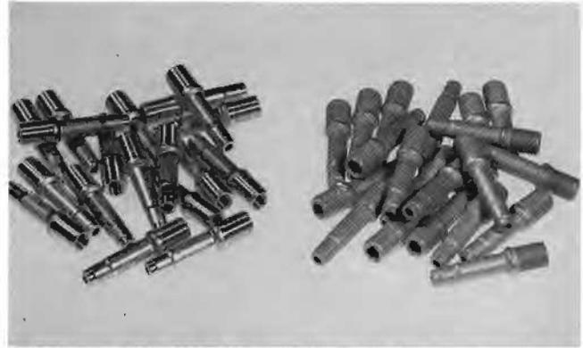
**Valve stems for tires are blast-treated with aluminum oxide before application of rubber coatings.**
