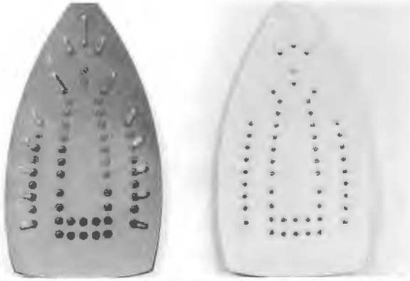
**Surface profiling of iron with silicon carbide improves adhesion of Teflon coating.**
