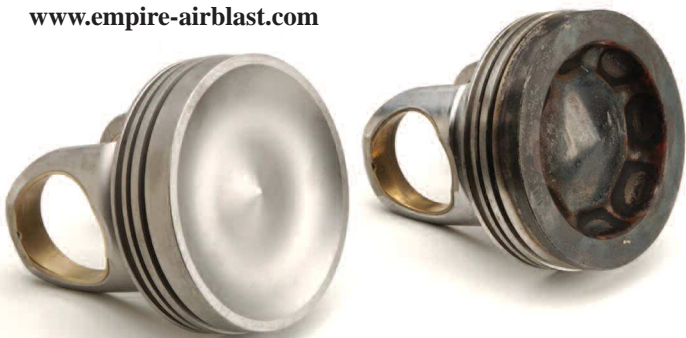
The correct mix of media and controls removes carbon deposits (right) without damaging base metals (left).
