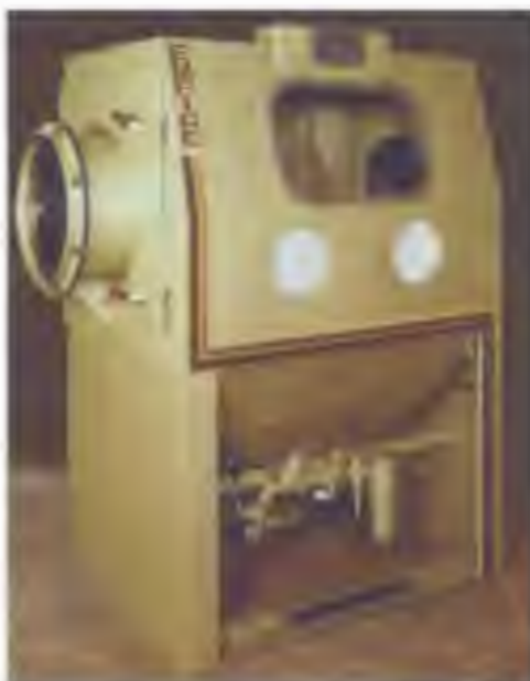
Figure 5. Pipe or other long, cylindrical parts can be finished using a compact cabinet equipped with baffled entrance and exit vestibules.
