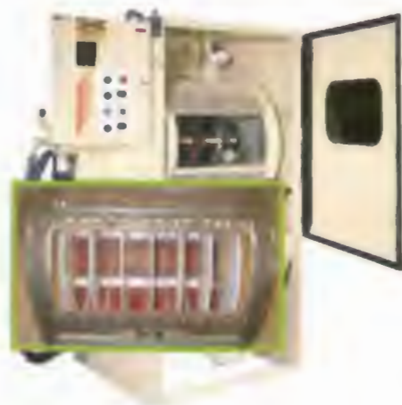
Figure 7. Modified basket blaster not only automates batch processing; it also protects workpieces from exposure to other metal surfaces.
