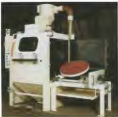
Figure 6. Tilting turntables provide easier access to heavier parts.
