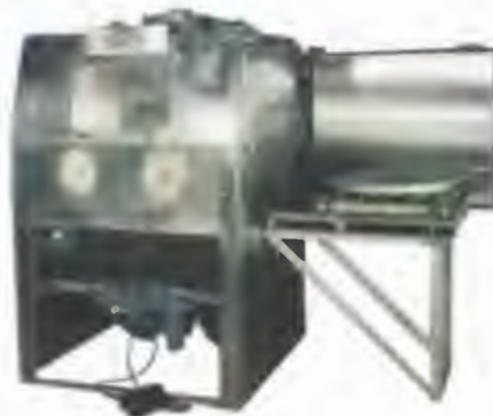
Figure 8. Stainless-steel construction reduces the chances of contamination from other types of steel.
