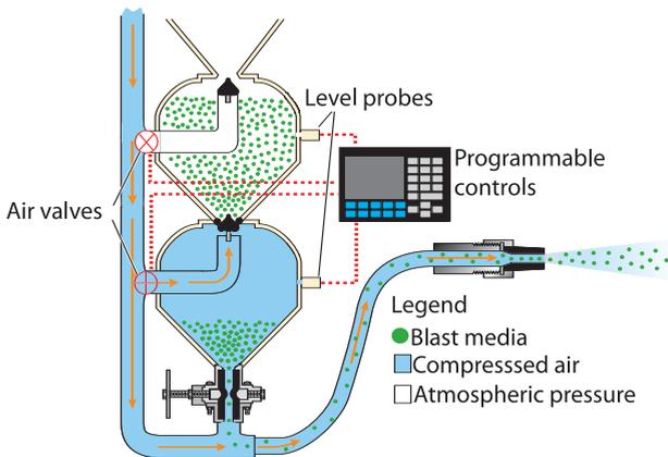
**Figure 3** Two-vessel system eliminates time outs for refills by coordinating pressurizations with media requirements. When the bottom vessel nears depletion, the top vessel pressurizes to supply more media via gravity feed.
