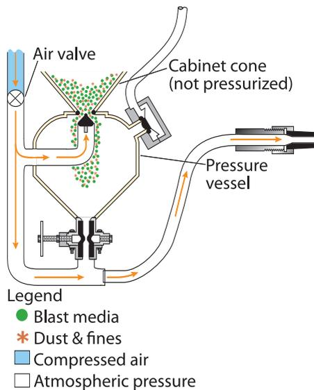
**Figure 1** If shot or abrasives are reused without being cleaned, broken media and work-surface debris degrade the mix progressively with each cycle, which wastes time and energy by slowing work and compromising quality. This drawing also shows why manual pressure-blast systems take time-outs. Because the media-supply vessel operates under pressure during blasting, it must be depressurized during refills. (Arrows show direction of air flow when system is active.)
