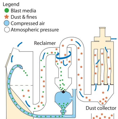
**Figure 2** Cyclonic reclaimers clean media by managing air flow. As air enters from the cabinet, it spirals in a downward vortex, throwing larger particles against the reclaimer's outer wall. Air pulled through the reclaimer's ports by the dust collector forms an upward counter vortex through a center tube that carries out dust and debris while good shot or abrasives drop into a storage hopper for reuse.
