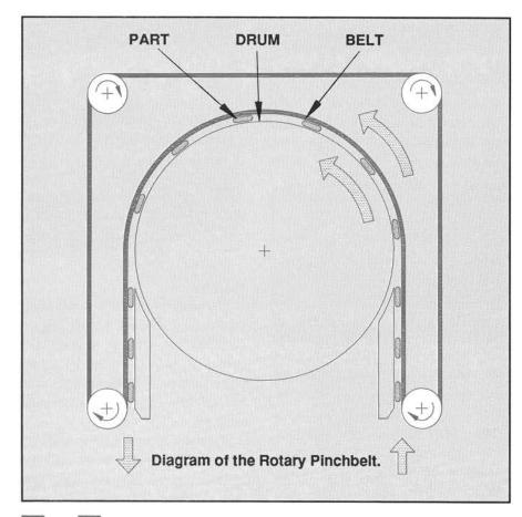
anufacturing hypodermic needles is a little less painful for two New England companies, thanks to a new concept in removing grinding burrs.
