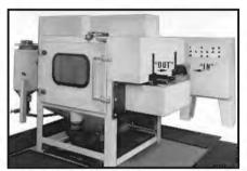
mechanism, which firmly suspends the strip of cannulas, exposing the downward facing cannula points. The workpieces pass over two upward facing blast nozzles which remove the burrs inside the heel of the ground cannula. Just one pass removes all burrs.
