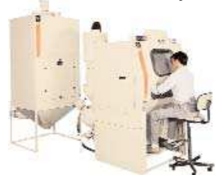
Figure 1: Industrial air-blast cabinets are available in a variety of standard configurations, including compact, easily transportable units that integrate blasting, media-reclamation, and dust-collection hardware within a single enclosure (left) and ergonomic models that improve operator efficiency over extended work periods (right).
