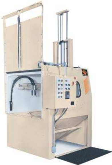
Fig. 5: Pressure-blast cabinet using plastic media combines a powered turntable with four nozzles, mounted on two linear oscillators, to strip wheels under the guidance of a programmable controller.
