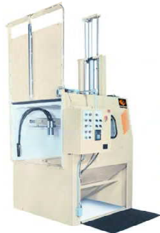
Figure 3 The blast cabinet shown borrows oscillating nozzles and a powered turntable from the automation shelf to expedite the cleaning of wheels. Programmable controls facilitate quick adjustment of part and nozzle movement.
