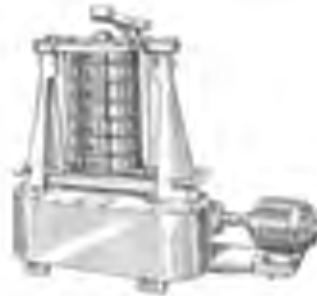
Figure 6: A stack of sieves, rotated and tapped automatically, segregate shot samples for inspection.
