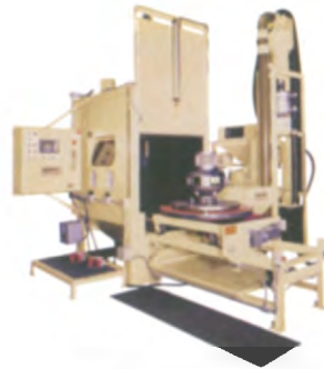
Figure 5: Programmable peening machine includes recycling equipment designed to assure consistent shot quality.
