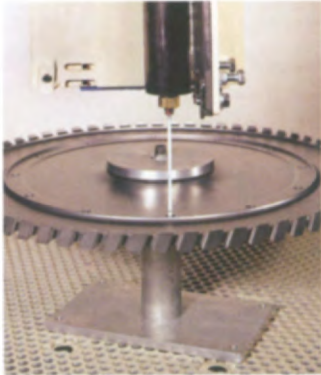
Figure 4: An oscillating lance, which diverts shot direction sideways, peens the interiors of holes and recessed areas.
