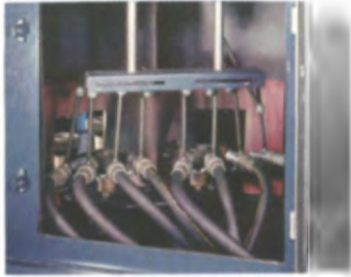
Figure 3: Multiple blast nozzles provide processing flexibility by targeting different areas and facets of work surfaces.
