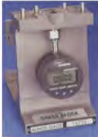
Figure 2: Modern Almen gauges provide precise readings of strip deflections used to measure peening intensity.
