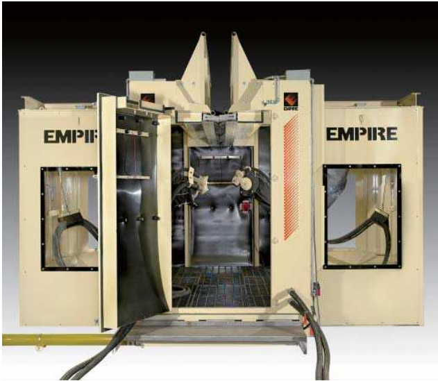
Nozzles mounted on dual robots to simultaneously process both sides of part with complex geometry
