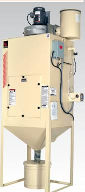
Standard Features: • Quick-release basket door • External blow-off gun • Door/blast interlock • Easily unloaded hopper door • Precision timer • 1/3-hp., DC variable drive (1 to 5 RPM) • 3-phase fan motor • Heavy-duty conveying hose • Tunable reclaimer • 1″ piping with general purpose filter, gauge and pressure regulator • Electrical control box • Two, 90-watt interior lights • Easily accessed media hopper • Observation window • Cabinet and dust-collector leveling bolts
