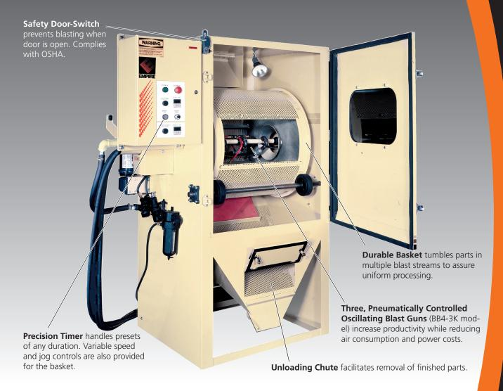
Empire's BB2 and BB4 Basket Blasters automate cleaning, peening and finishing of small workpieces. With certain types of parts, no other finishing method can compare to these heavy-duty production machines in terms of speed and quality results.
