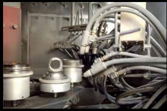
Indexing Turntable Machine coordinates 16 blast guns, oscillating vertically and horizontally, with rotating work stations to assure thorough cleaning in a single pass.
