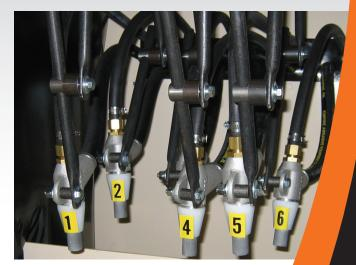
**Six or Four Blast Guns** mounted on separately adjustable holders enable operators to control blast coverage.
