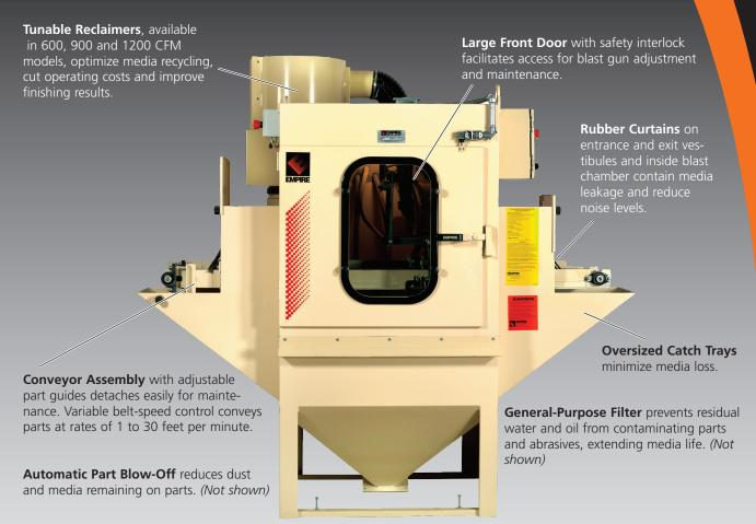
Based on Empire's field-proven Pro-Finish® technology, the IL-885 incorporates a rugged conveyor assembly driving a 9-inch-wide by 72-inch-long belt. Variable speed controls and adjustable parts guides provide the versatility to deburr, clean, profile and finish parts of many different shapes and sizes ranging from tubular to flat; if two sides of a workpiece require blasting, the piece can be reloaded for a second pass.
