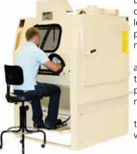
Designed for sit-down blasting, these ergonomic cabinets include a padded armrest, an elevated foot rest for treadle control, top-entry piping for less arm stress, a sound dampener to reduce noise and a front mounted pressure regulator — all aimed at improving operator comfort and performance during long, repetitive blast cycles.
