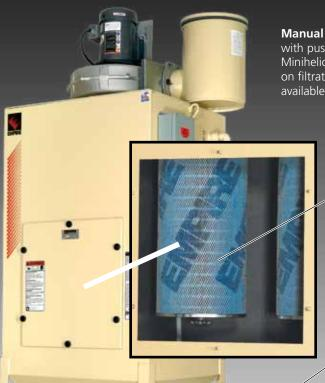
Manual Reverse Jet-Pulse Dust Purging can be performed with push-button ease while the air-blast system is operating. Minihelic gauge keeps operator informed about dust buildup on filtration surfaces. A fully automatic photohelic control is available as an option.
